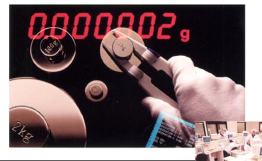
recision weights slip out of tolerance for many reasons: improper handling, a scratch, a nick, a friction wear, a trace of environmental contaminant such as oil or grease... or just plain old dust and dirt. To protect the accuracy of your weighing work,
