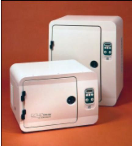
The Models IN30 and IN40 are not programmable. They are simple set-and-forget models. Set the temperature and the unit will go there. To change temperature, simply key in another target. The units are bench top in size. The IN30 has 27.5 liter capacity and the IN40 has 55 liter capacity. Both have a temperature range from 4.0°C to 70.0°C. They have seamless, white ABS plastic chambers with capped holes in the left side of the sheet metal case for routing cords for shakers or tubing
