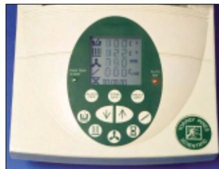
*Above is a close-up of the membrane switch and display. To set a solution temperature, press the solution icon and then the UP arrow until the desired temperature is displayed. The instrument does the rest. Plate temperature, temperature ramping, stirring speed, and timer are just as simple to set.*
