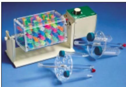
using a simple knob control. The unit is provided with a mounting rack that holds 50-0.5 ml centrifuge tubes and 48-1.5ml centrifuge tubes. Accessory racks can be ordered that hold 16-15ml tubes or 6-50ml tubes. Changing from the provided rack to accessory racks can be done in just minutes. The rod holding the racks is easily removed for changing from one rack to another.
