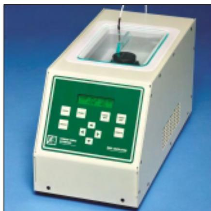
The Model CB20 is a Peltier-based chilling/heating constant temperature small volume circulator with a temperature range from 4.0°C to 70.0°C. It can circulate up to 300 ml/minute of solution from a 1000ml reservoir for controlling the temperature of small remote samples like
