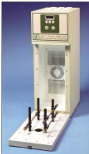
very reliable. It has a very large chamber measuring 15.5" (39.37 cm) high x 6.385" (16.28 cm) wide x 5.125" (13.02 cm) deep. The chamber will easily hold 4-30 cm x 1" columns and a Rheodyne valve. Chamber temperature uniformity is  $\pm 0.5^{\circ}\text{C}$ .
