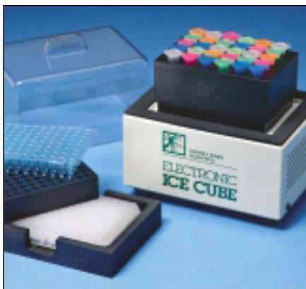
The Model IC10, called the Electronic Ice Cube, is an uncontrolled, Peltier-driven chilling device that chills only. It will go to 30°C below room temperature. The unit is designed to replace an ice bucket. No more water, mess or changing ice as it melts. The unit has the same size chilling plate as all the other units in this section and uses all the same sample blocks and covers. It is very small and uses virtually no bench
