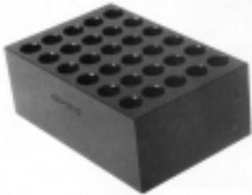
The block at the left is number 620-5013 and is for 30-1.5 ml. centrifuge tubes. The block measures 4.375 in. (11.11 cm.) long by 3.0 in. (7.62 cm.) wide by 1.75 in. (4.45 cm.) thick. All blocks are precision machined from solid aluminum to exactly fit the tube shape and black anodized for better heat transfer and protection from spills. The bottom of the blocks are machined to “nest” on the plate to prevent movement. Also, custom blocks for any sample container can be made upon request.
