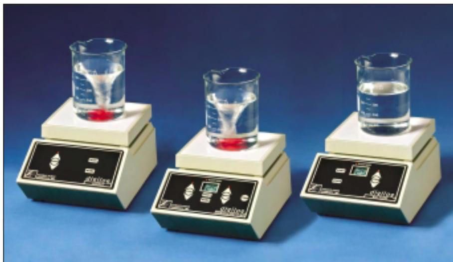
Three models of DigiLog units are available: a hot plate Model HP20, a stirrer Model ST20 and a stirring hot plate Model HS20. All use the same compact, rugged cast aluminum chassis that is designed to keep spills out of the case. All controls are mounted forward of the heater plate for safety. All electronic controls are on one simple PC board, and all controls have red indicator LED's that illuminate when activated.
