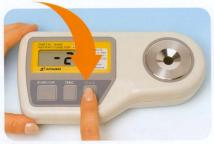
Press the SCALE switch to display and select a measurement scale.
