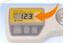
The measurement scale blinks two times on the LCD, and then the measured value of the sample is displayed on the LCD.
