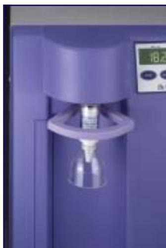
Filter 0.2 micron with Filling Bell
