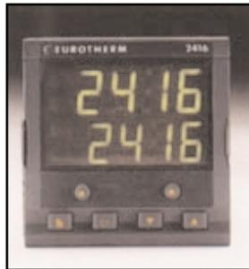
Other Options Additional control systems can be supplied and they include cascade control, multi-segment programmers and process timers. The Carbolite 201 controller is also available with an integral process timer. When the working setpoint is reached, a timed period starts and can either end with an audible alarm or to switch off the power at the end of the time period.
