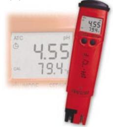
The pHep<sup>®</sup>'s replaceable electrode has a pull-out cloth junction. When the cloth junction becomes dirty from routine testing, simply pull out 3 mm (1/8") to rejuvenate the electrode.
