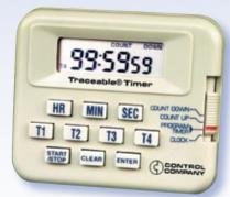
Timer operates on all channels simultaneously; it has five countdown channels, a stopwatch channel, and a time of day channel. Counts both up and down to 99 hours, 59 minutes, 59 seconds. Accuracy is 0.01%. Unique "thru-zero" feature allows counting down, alarming, and counting up. A time-out mode stops the timer for "off" periods in both up and down timing. T1 through T4 may be started simultaneously or individually.
