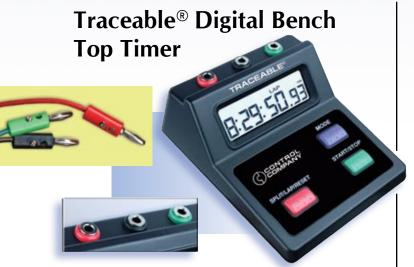
The perfect size—has a large-screen LCD and a small, labbench footprint. Times up from 0.01 second to 9 hours, 59 minutes, 59 seconds, and 99 hundredths of a second. Switchable between cumulative and interval-split, the unit also allows an infinite number of time-outs. Oversize buttons make it easy to use. Three 4mm sockets (and supplied test leads) allow external triggering of the Start/Stop and Split/Lap/Reset functions of the timer. Digital display is ¾-inch-high and is readable from 10 feet.
