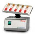
The Thermo Scientific Multi-Tube Rotator has a fixed shaker speed. The circular motion coupled with a rocking pattern keeps liquids and solutions mixed gently without the potential for shearing or other damage.
